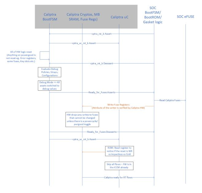
**Note:** Since Caliptra IP may be placed in a "S5" domain of the device, there may be devices where Caliptra IP may not go through reset on a device hot reset or CPU warm reset. But the flow shows what happens when such a reset happens.
